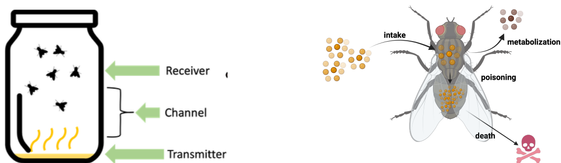
Figure 1: Left: Synthetic MC system involving living insects. Transmitter: Evaporation of toxic signaling molecules (fumigants); Channel: Sealed chamber; Receiver: Swarm of insects. Right: Schematic illustration of the signaling molecule uptake by the insects. Signaling molecules are either accumulated, leading to death of the insect, or metabolized into biomass.
